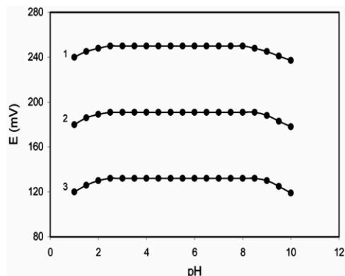
Fig.-3 The effect of pH of the test solution on the potential response of the perchlorate-selective electrode at three different  $\text{ClO}_4^-$  concentrations: (1)  $1.0 \times 10^{-4}$  M (2)  $1.0 \times 10^{-3}$  M, (3)  $1.0 \times 10^{-2}$  M
